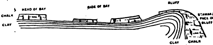
Diagram of Chalk Bluff, showing the mass of clay immediately behind it and the discontinuous line of chalk masses round the Bay.
